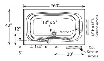
Product Shown: Signa™ 5 Whirlpool Bath with 3 Tile Flange Right Hand Model: D560 \* Measurements inside unit represent cutout in floor to allow for drain/overflow. Minimum Service Access dimensions given.
